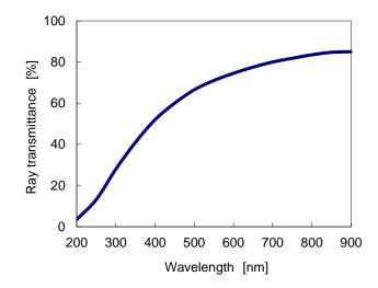
Figure 17: UV-VIS Spectrum of KF Polymer (KF POLYMER #1000, Film thickness: 100 μm)
