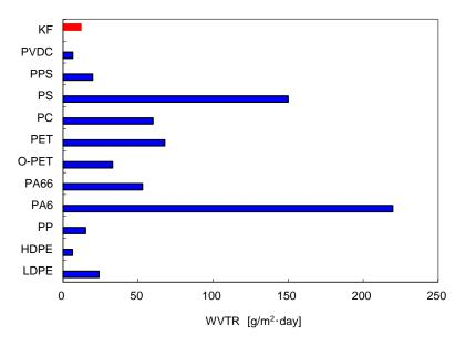
Figure 15: WVTR of KF POLYMER and other polymers (Film thickness: 20 µm, 40°C 90 %RH)
