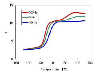
Figure 12: Dielectric constant (KF POLYMER #1000)
