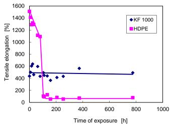
Figure 14: Tensile elongation of KF POLYMER after ozone exposure
