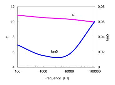
Figure 11: Dielectric constant and Frequency dispersion (KF POLYMER #1000) at 23°C
