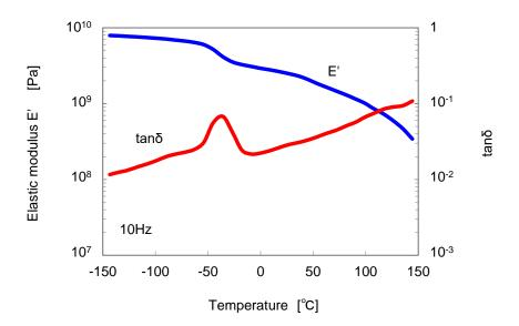
Figure 8: Viscoelasticity (KF POLYMER #1000)
