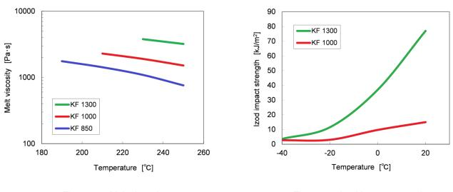
Figure 6: Melt viscosity
