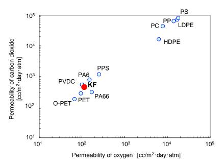
Figure 16: O<sub>2</sub> and CO<sub>2</sub> permeability of KF POLYMER and other polymers (Film thickness: 20 µm, 30°C, 80 %RH)
