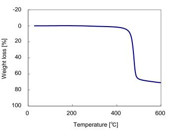
Figure 10: Thermogravimetric analysis (KF POLYMER #1000)
