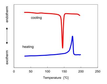
Figure 9: The behavior of melting point and crystallization point (KF POLYMER #1000) (Heating or cooling rate:  $10^{\circ}$ C /min in N<sub>2</sub>)
