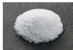
Polyvinylidene fluoride (PVDF) PVDF is a super engineering plastic with an excellent balance of chemical resistance and moldability, used in such fields as electronic materials and water treatment membranes.
