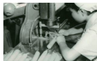
Sausage ligature process using a stamping machine
