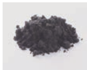
Hard carbon anode materials for lithium-ion batteries ( Cabotron )
