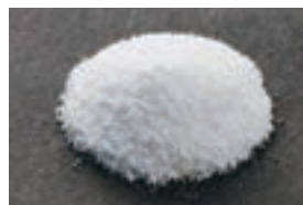
PVDF used as a binder for lithium-ion batteries
